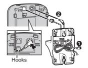
Insert the hooks on the wall mounting adaptor into holes (a) and (b) on the base unit.
