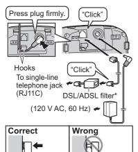
\*DSL/ADSL filter (not supplied) is required if you have DSL/ADSL service.
